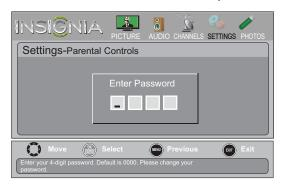
**4** Press the number buttons to enter the four-digit password. The *Settings-Parental Controls* menu opens with **Button Lock** highlighted.
